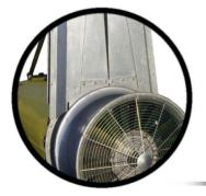
THE MUNCKHOF TOWERS ARE DESIGNED TO EVENLY DISTRIBUTE AIR FLOW THROUGH OUT THE ENTIRE HEIGHT OF THE CANOPY PLACING SPRAY MATERIAL ONLY WHERE IT IS NEEDED.
