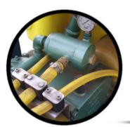
MUNCKHOF 1000 LT SPRAYERS USE A POWERFULL 70 LT/MIN PLUNGER PUMP WITH THROUGH PTO FOR FAN DRIVE.
