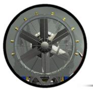
A LARGE 610MM FAN PROVIDES A POWERFUL AIRSTREAM FOR SENDING MATERIAL THROUGH THE ENTIRE CANOPY, A BELT DRIVE IS USED TO REDUCE SHOCK LOADS ON THE DRIVE-TRAIN
