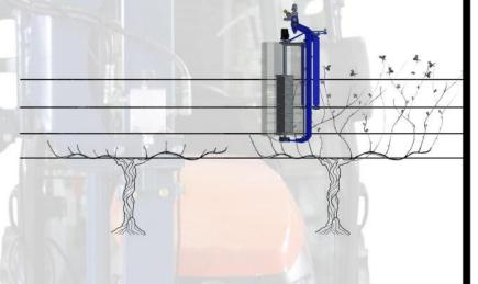
The Pre Pruner not only cuts the vast majority of unwanted wood, it also breaks the wood down and strips it from the canopy. There is no need for pulling out of canes, and it eliminates the tangled mass on the vineyard floor.
