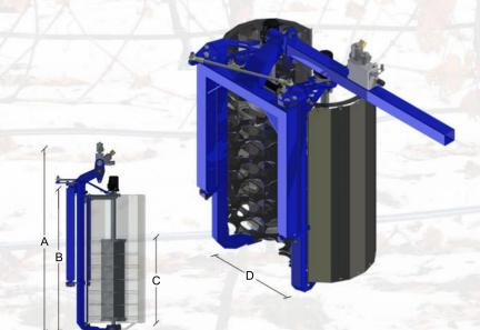
The short stack pre pruner is designed for use in VSP plantings, and works best with cane pruned training styles. The total pre pruner height is 51" (E). The column has 20" of cutting depth (G), and a 32" tall opening (F). This gives ample space for overhead irrigation. A 21" wide mouth (H) makes this machine capable of handling small T-bars.
